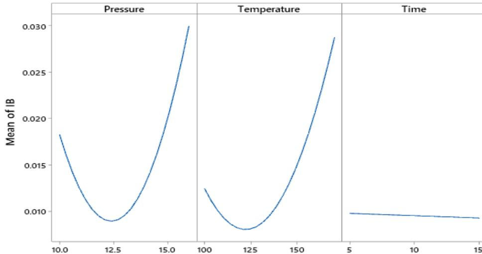
Fig. 5 - Main effects plot for IB of binderless boards manufactured from Abura sawdust
