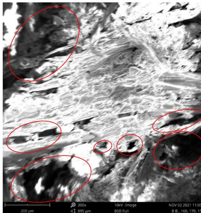
Fig. 6 - SEM of bioboards produced at 16 MPa, 170°C and 15 minutes for magnifications of  $\times 300$  (with voids highlighted)
