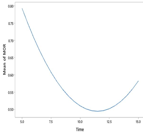
Fig. 4 - Main effects plot for MOR of binderless boards manufactured from Abura sawdust
