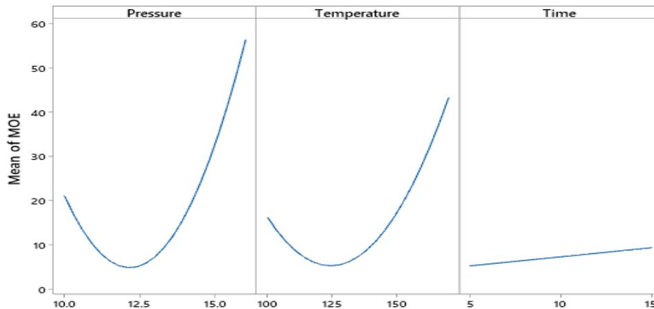
**Fig. 3 - Main effects plot for MOE of binderless boards manufactured from Abura sawdust**
