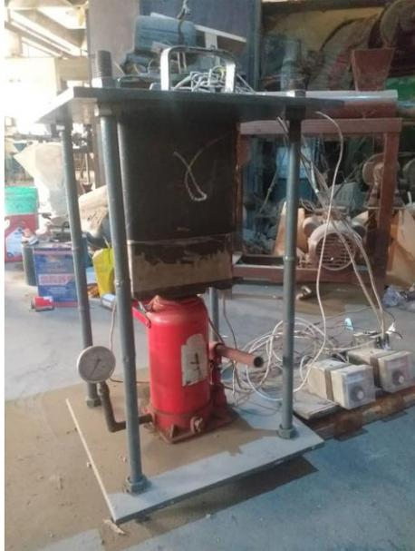
Fig. 1 - Laboratory scale hot-press developed for manufacture of bioboards
