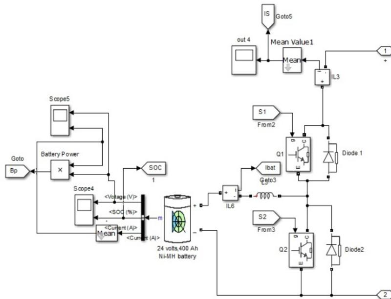
**Fig. 6 - Battery and DC-DC converter system**
