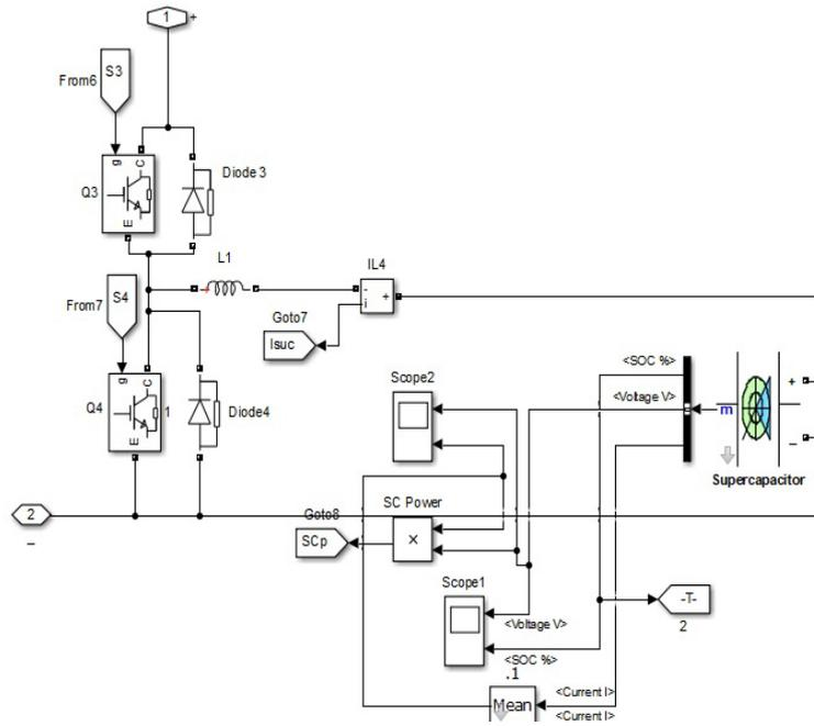
**Fig. 7 - Supercapacitor and DC-DC converter system**
