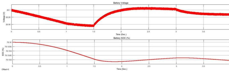
Fig. 14 - Battery voltage and battery SOC waveform
