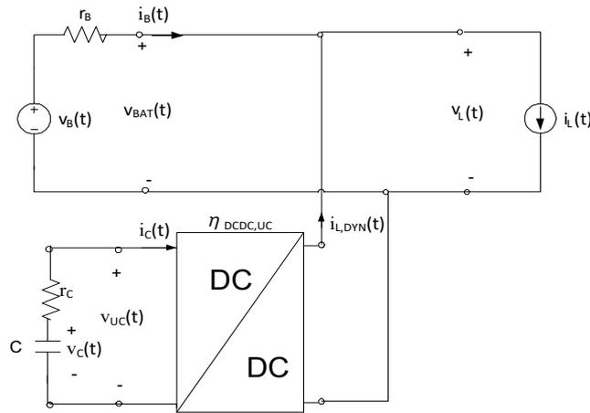
Fig. 2B - DC-DC converter connected with SC
