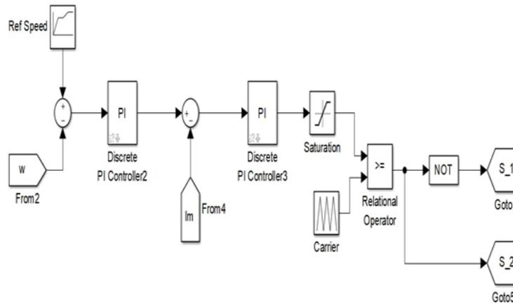
**Fig. 9 - Motor PWM speed control**
