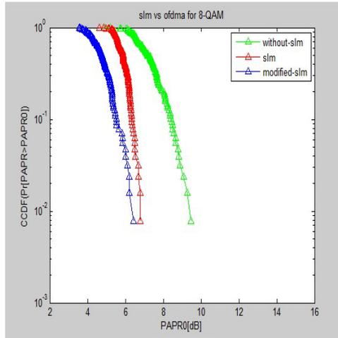
**Fig. 12 - PAPR improvement in modified SLM over conventional OFDM and SLM for 8-QAM**
