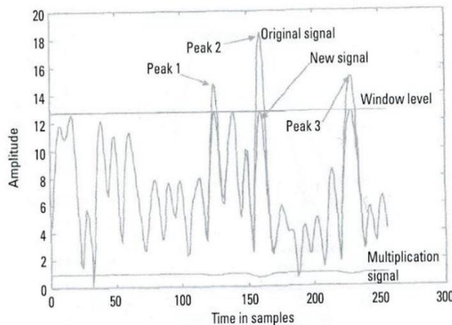
**Fig. 4 - Windowing an OFDM time signal**
