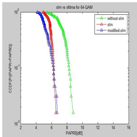
**Fig. 13 - The performance of PAPR in OFDM without SLM, with SLM and Modified SLM using 64-QAM modulation**
