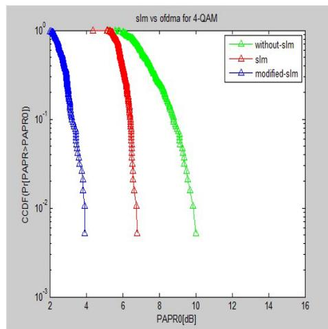
**Fig. 11 - PAPR improvement in modified SLM over conventional OFDM and SLM for 4-QAM**
