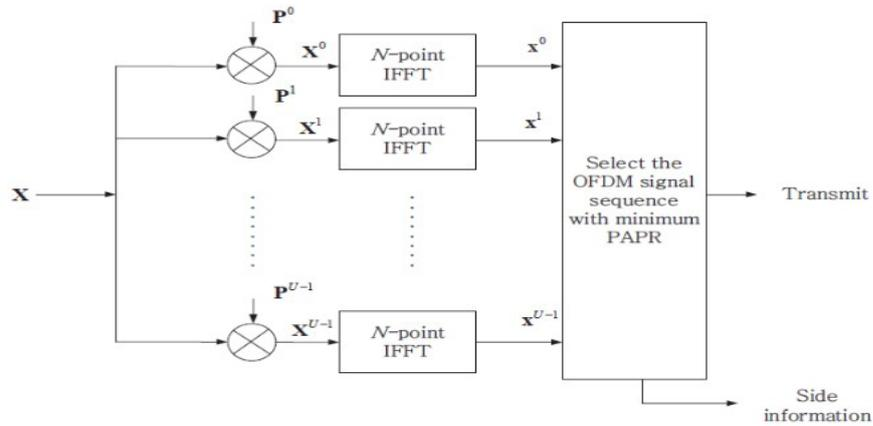
Fig. 8 - The conventional SLM method
