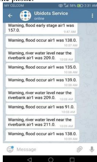
Fig. 9 - Ubidots notification to users on flood occurrence
