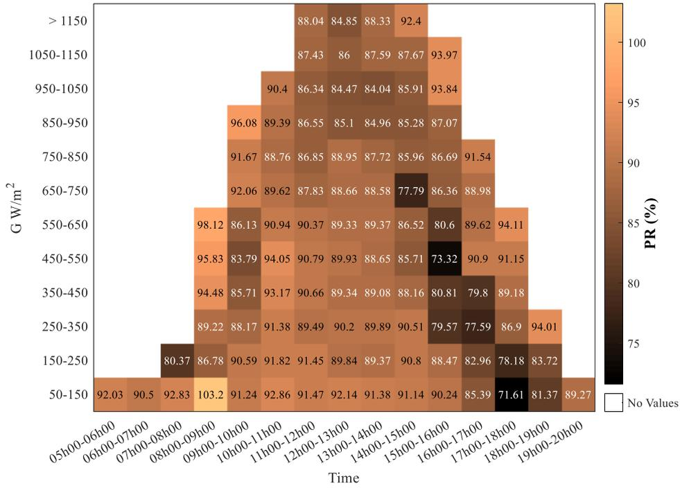
Fig 5 - PR (%) and G (W/m<sup>2</sup>) versus Time in 80 days
