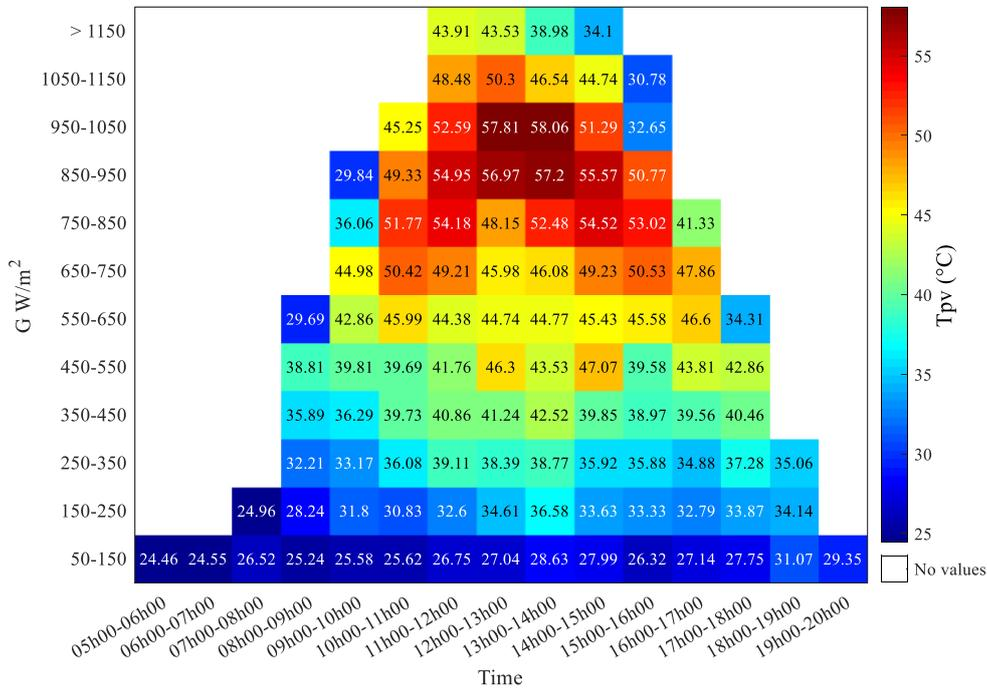
Fig 6 - Tpv (°C) and G (W/m<sup>2</sup>) versus Time in 80 days
