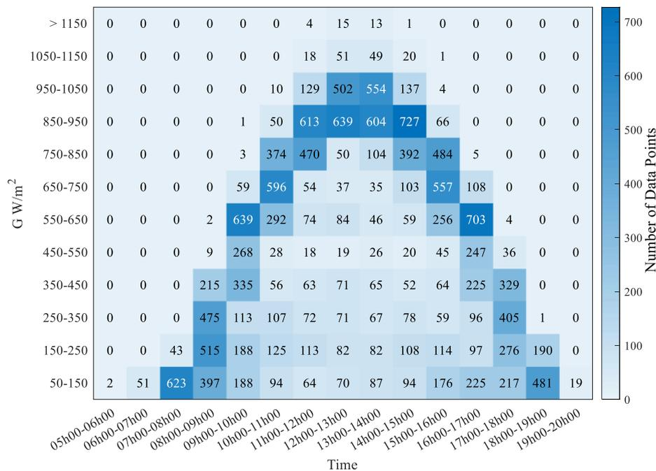
**Fig 4 - Number of data points and G (W/m<sup>2</sup>) Versus time in 80 days**
