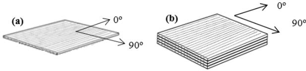
Fig. 2 Composite, (a) lamina, and (b) laminate.
