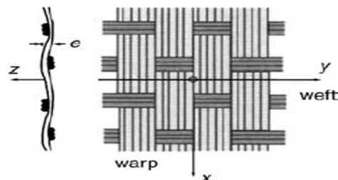
Fig. 3 Warp and weft direction of woven fabric [39].
