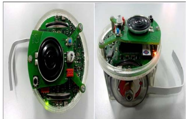
Fig. 3.2 The top view and the side view of the L-shape object gripper with a dimension of 4cm × 4cm attached at the back of the E-puck robot.
