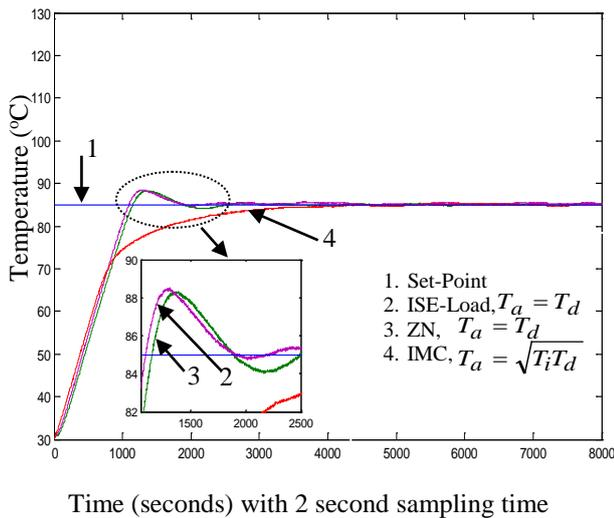
Fig. 11 Comparative real time performance of PID controller with difference tuning: ISE –Load with  $T_a$  equal to  $T_d$ , ZN with  $T_a$  equal to  $T_d$  and IMC with  $T_a$  equal to  $\sqrt{T_i T_d}$ .
