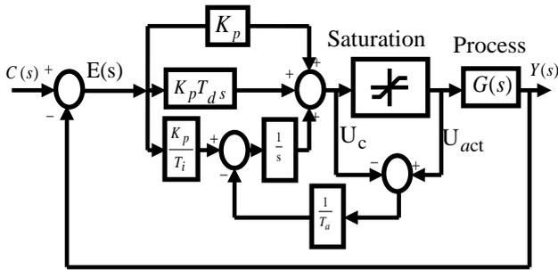
Fig. 6 PID controller with back calculation anti windup block diagram.
