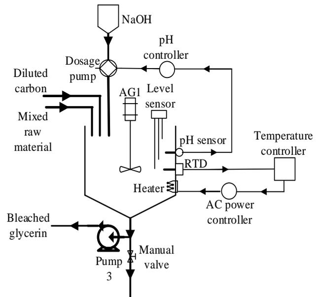
Fig. 2 P&ID of reactor tank for glycerin bleaching process.
