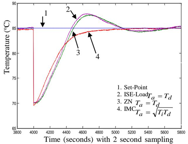
Fig. 12 Comparative real time performance of PID controller with difference tuning: ISE –Load with  $T_a$  equal to  $T_d$ , ZN with  $T_a$  equal to  $T_d$  and IMC with  $T_a$  equal to  $\sqrt{T_i T_d}$  on disturbances recovery.
