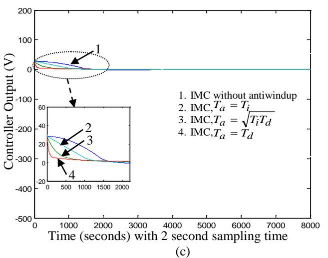
Fig. 7 Performance response of PID controller with and without antiwindup with different tracking time constant; (a) ISE-Load, (b) ZN, (c) IMC.
