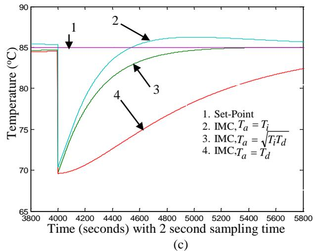
Fig. 9 Behavior of Integral term of PID controller with and without antiwindup with different tracking time constant; (a) ISE-Load, (b) ZN, (c) IMC.
