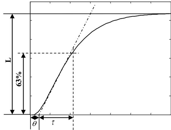
Fig 5 Tangent and point method in determination process parameter
