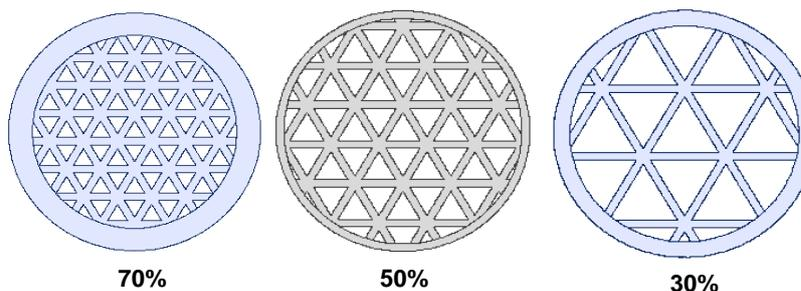
**Fig. 2 - Different infill density structures for the sample**
