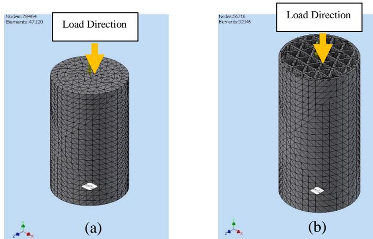
Fig. 4: Meshing density and load direction (a) surface structure of triangular pattern at 50% density and (b) internal structure of triangular pattern at 50% density
