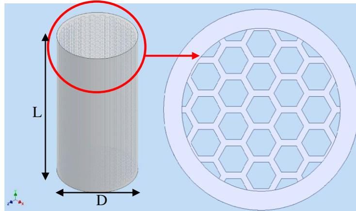
Fig. 3 - Internal hexagonal structure design
