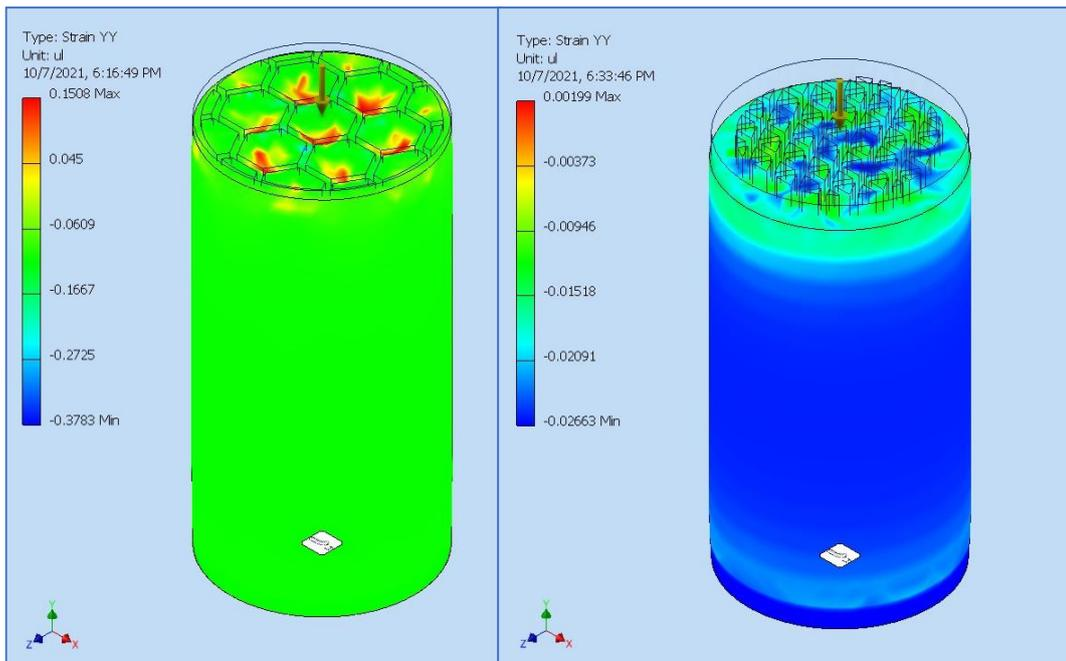
**Fig. 5 - Compressive strain result for samples 3 (left) and 8 (right)**
