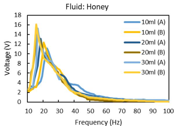
**Fig. 13 - Operating frequency for honey in both containers**
