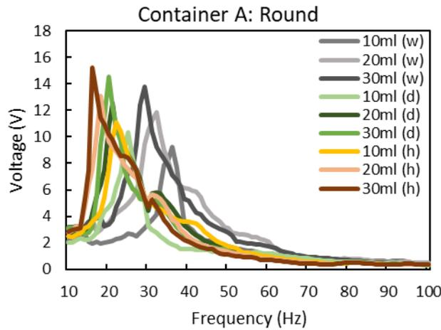
Fig. 9 - Operating frequency for round container
