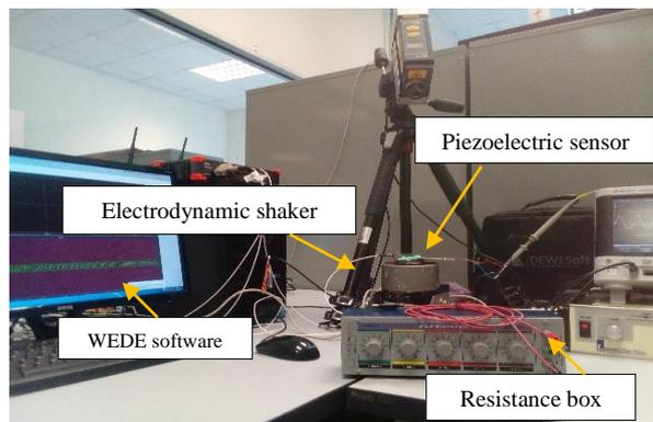
**Fig. 2 - Experimental setup 1**
