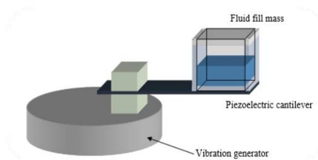
**Fig. 3 - Experimental setup 2**
