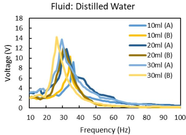
**Fig. 11 - Operating frequency for water in both containers**
