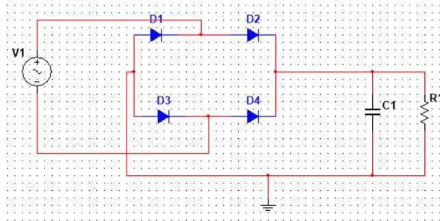
**Fig. 6 - Full-wave bridge rectifier circuit**
