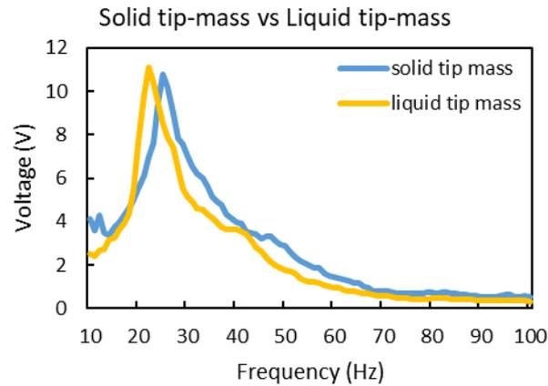
Fig. 14 - Voltage-Frequency characteristics of solid tip mass and liquid tip mass
