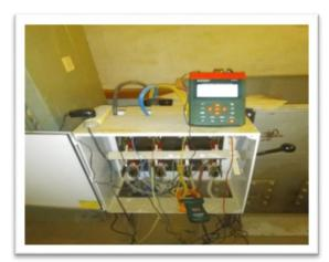
Fig.4 - PHA measurements Setup
