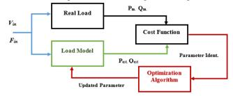
Fig. 2 - The procedure of load modeling and identification
