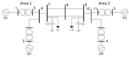
Fig. 6 - 2 - Area 4- Machine Kundur test system
