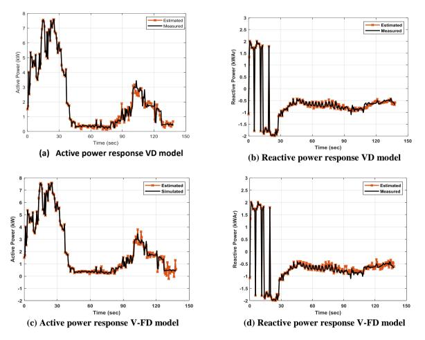
Fig. 9 - Active and reactive power responses of VD and V-FD models of training
