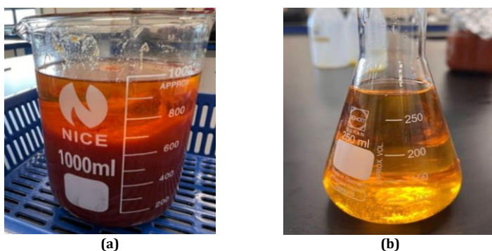
Fig. 1 One-step transesterification process of WCO into BD
