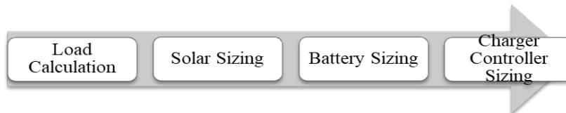
Fig. 2 - The procedure for measuring an important component in the installation of solar panel
