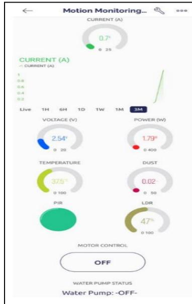
**Fig. 14 - The interface of the solar monitoring system through the Blynk application**
