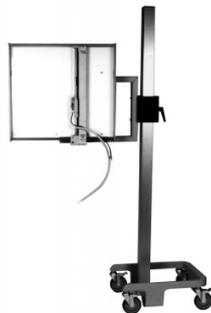
Fig. 3 - Mobile contour plotter [17]
