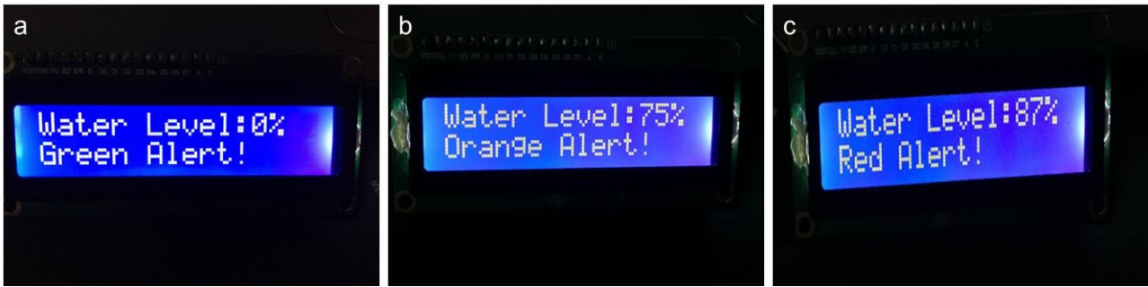
Fig. 12 - LCD Display for (a) safe level green alert; (b) cautious level orange alert and; (c) danger level red alert
