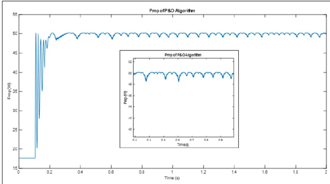
**Fig. 11 - Maximum power point using P&O algorithm**
