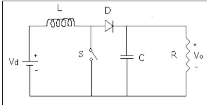
Fig. 4 - Boost converter circuit [19]
