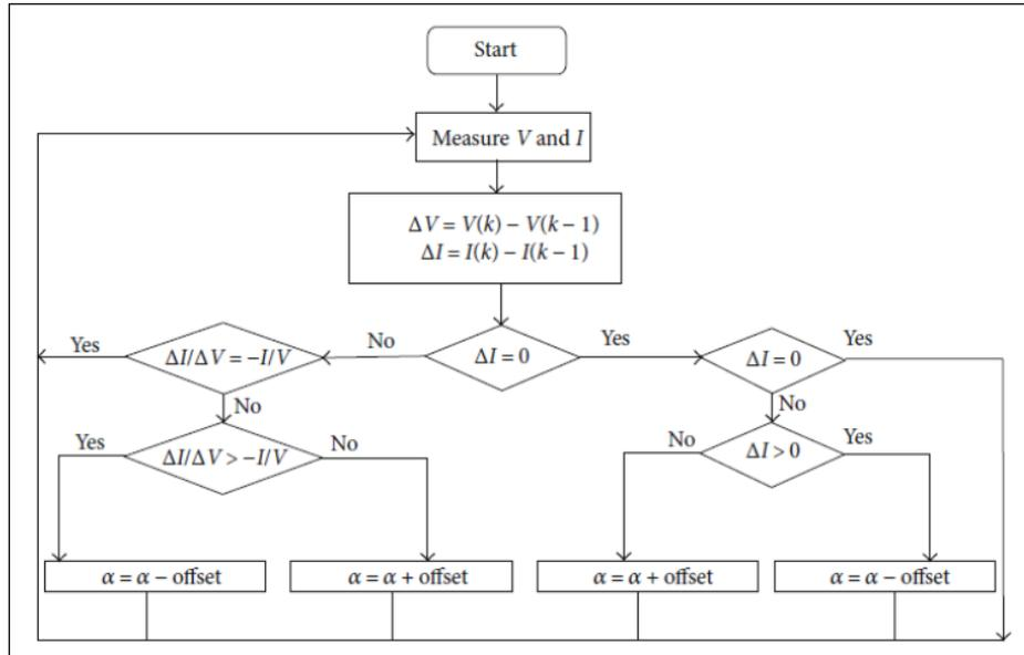
Fig. 6 - Flow chart of conventional InC algorithm [21]
