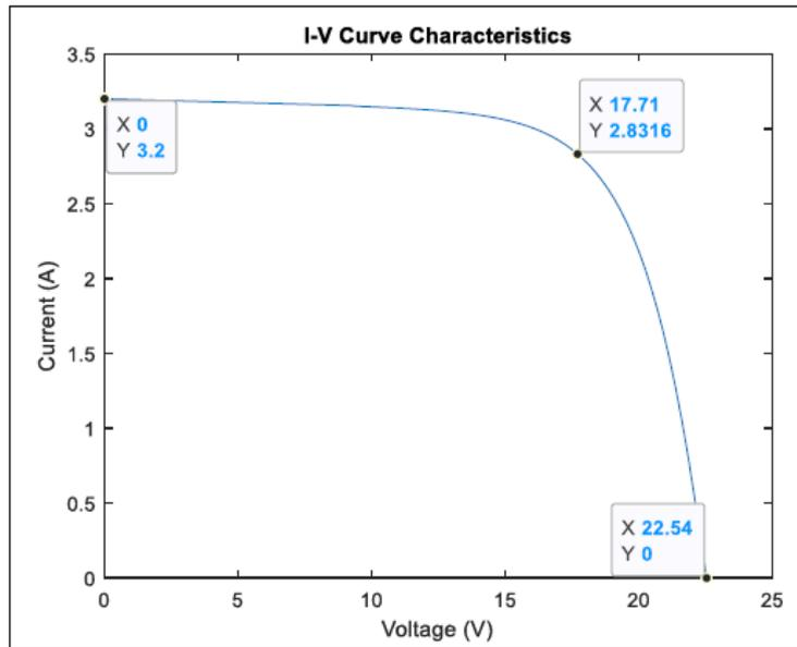
**Fig. 9 - Current versus voltage curve characteristics of PV module**
