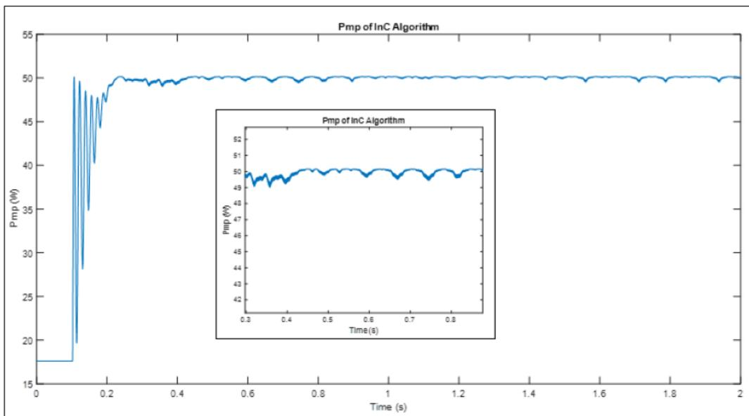
**Fig. 12 - Maximum power point using InC algorithm**
