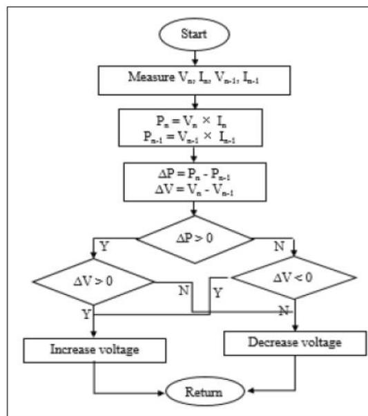
Fig. 5 - Flow chart of conventional P&O algorithm [20]
