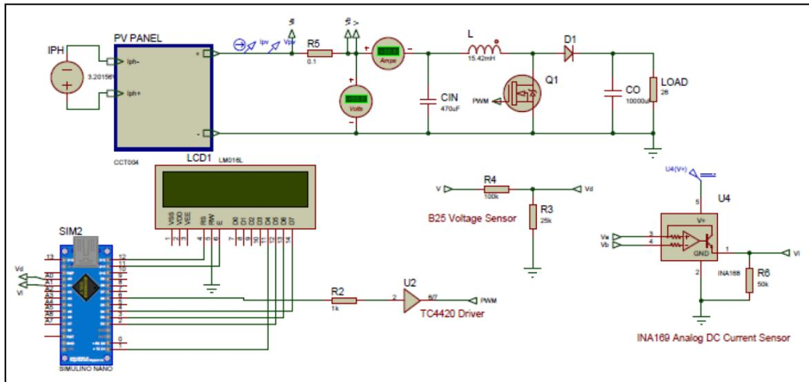
**Fig. 8 - Modified MPPT charge controller by using Arduino NANO**
