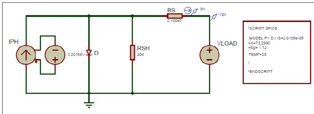
Fig. 7 - PV Module using SPICE in Proteus [11]
