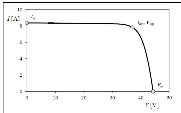
**Fig. 3 - Characteristic I-V Curves of a Solar Panel [16]**
