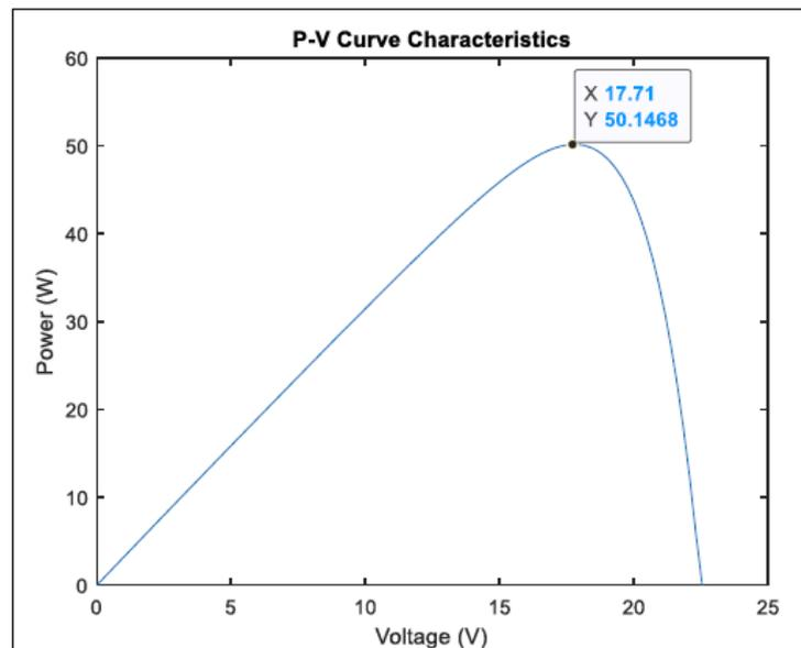
**Fig. 10 - Power versus voltage curve characteristics of PV module**
