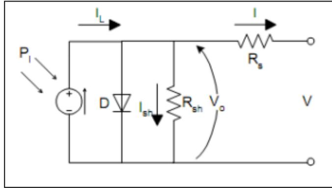
**Fig. 2 - PV module electrical circuit equivalent [14]**
