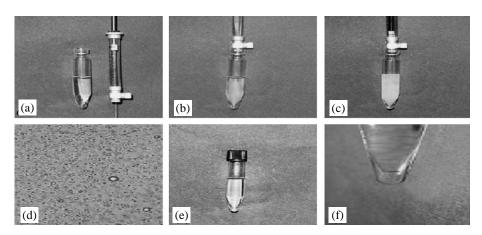
Figure 1: Overall procedure of DLLME technique to extract PAH from sample [17].
