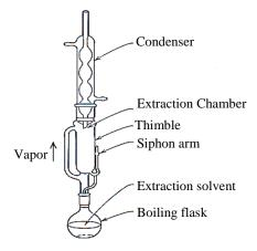
Figure 4: Soxhlet Extractor [14].
