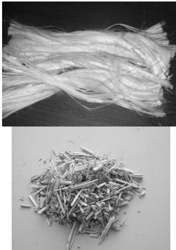
Figure 3: Kenaf bast (left) and grounded kenaf core (right)
