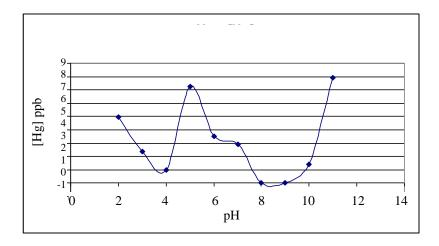
Figure 11: Effect of pH on Membrane Separation with Pretreatment
