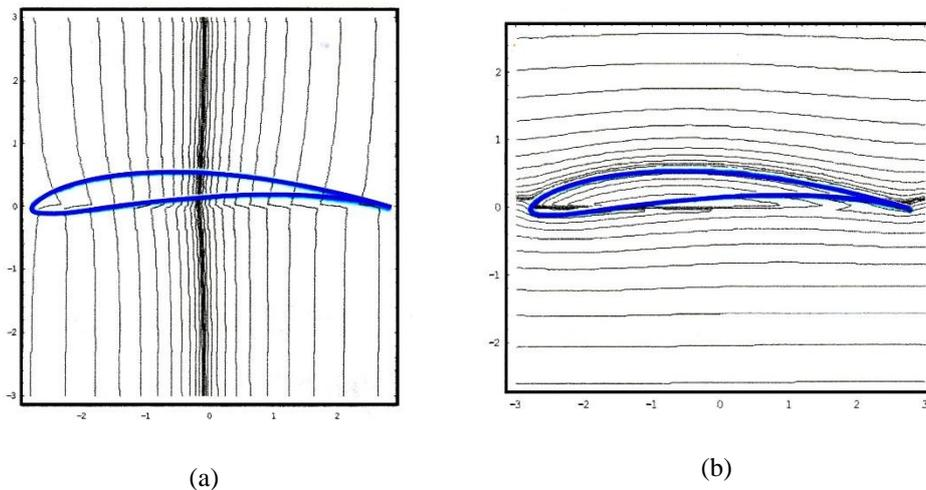
**Fig. 2 - Joukowsky airfoil with (a) equipotential lines and (b) streamlines lines**
