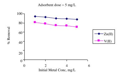
Figure 2: Effect of initial metal concentration on percent removal of heavy metals by silica aerogel.
