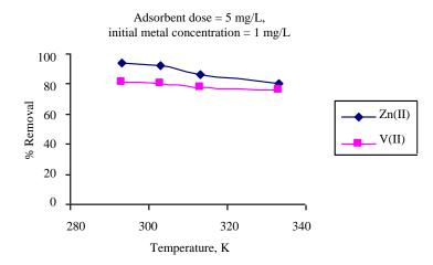
Figure 4: Effect of temperate on percent removal of heavy metals by silica aerogel
