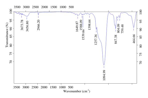
Figure 1: FT-IR spectra of silica aerogel powder
