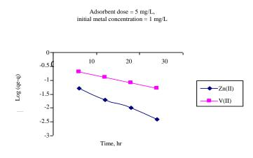
Figure 6: Plot for Lagergren rate constant for adsorption of heavy metal ions by silica aerogel.
