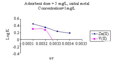
Figure 5: Plot of log Kc and 1/T for heavy metals on silica aerogel.
