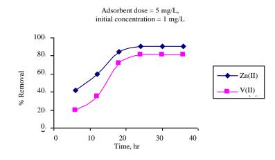
Figure 3: Effect of contact time on percent removal of heavy metals by silica aerogel.
