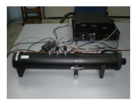
Figure 2: The impedance tube gadget for acoustic analysis
