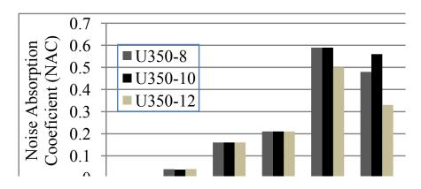
**Figure 5**: Sound Absorption Coefficient versus Frequency of Kenaf Core Particleboard at Density of 350 kg/m<sup>3</sup> with different UF loading
