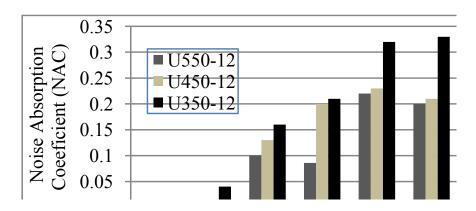
Figure 8: Sound Absorption Coefficient versus Frequency of Kenaf Core Particleboard at UF Loading of 12% and Variable Board Density
