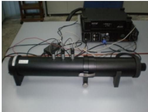
**Figure 2:** The impedance tube gadget for acoustic analysis
