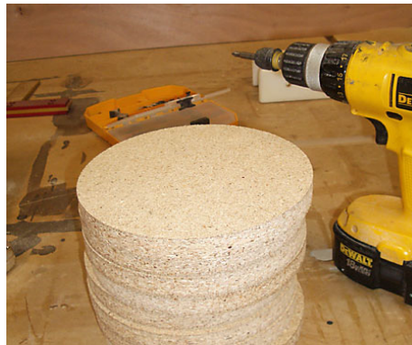
Figure 1: The circle shape of kenaf particleboard for NAC test
