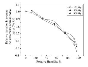
Figure 8: Influence of pre-irradiation RH conditions on dose response at different temperatures
