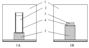
1→Irradiation volume of GC – 900, 2→ Fricke dosimeter, 3→ Glycine pellet, 4→ Build-up, 5→ Perspex spacer placed on a cylindrical perspex base
