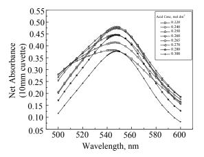
Figure 4: Effect of acidity on dose response at different wavelengths
