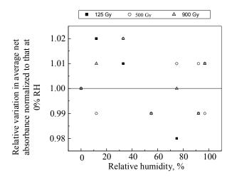
Figure 9: Influence of relative humidity conditions during irradiation on dose response
