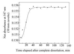
Figure 6: Net absorbance change after dissolution of glycine pellet in FX
