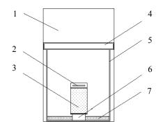
1→Irradiation volume of GC 900, 2→ Glycine pellet in dosimeter container, 3→ Perspex spacer, 4→ Lid of container, 5→ Plastic container, 6→ Perspex jig, 7→ Saturated salt solution
