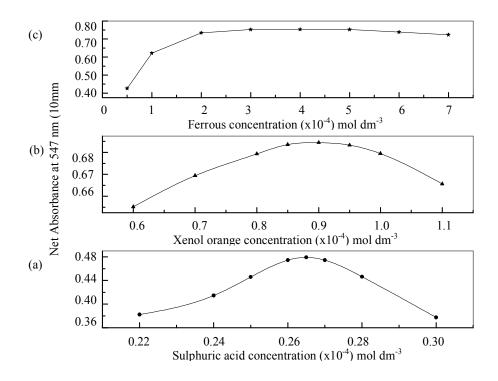
Figure 5: Optimum FX composition: (a) Dose response at different sulphuric acid concentration, (b) Effect of xylenol orange concentration on dose response, (c) Effect of ferrous ion concentration on dose response.
