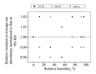
Figure 10: Influence of relative humidity conditions prevailing at post-irradiation storage of pellets
