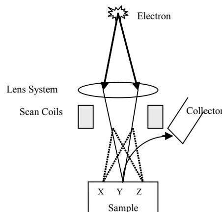
Figure 5. Schematic operating principle of a scanning electron microscope.
