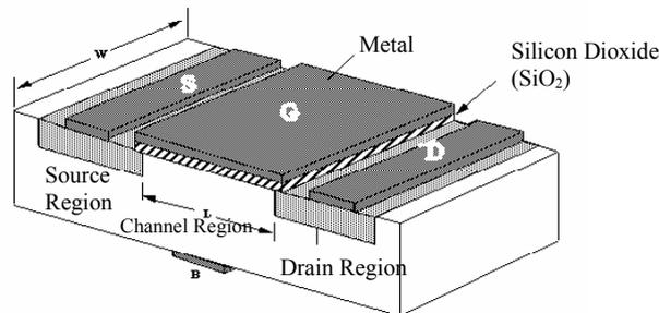
Figure 1. A typical MOSFET structure.
