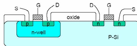
Figure 4. CMOS structure that consists of NMOS and PMOS on the same substrate.
