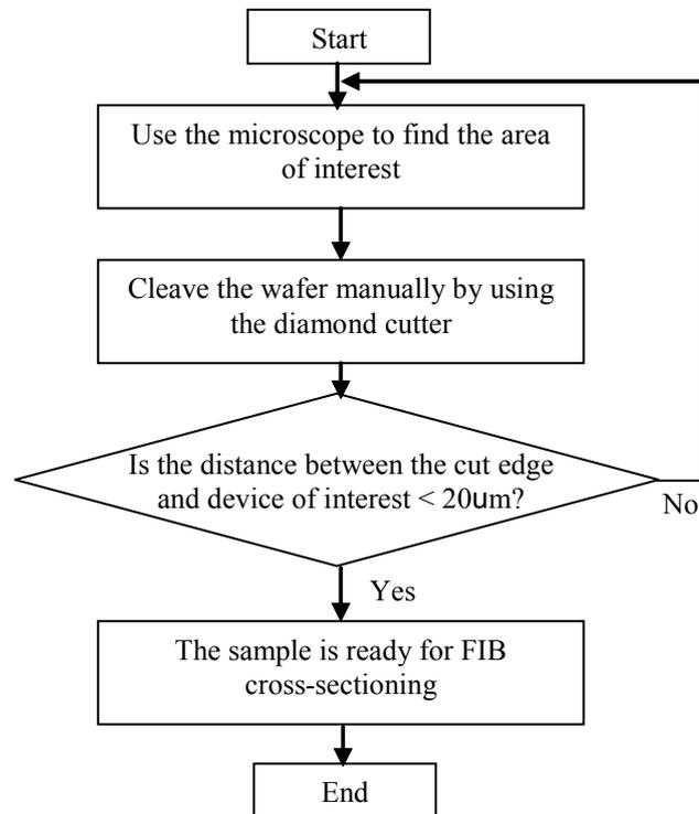
Figure 6. The flow chart of steps wafers cleaving.
