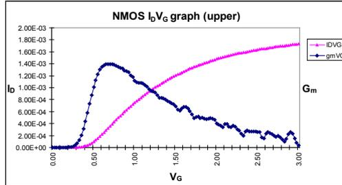
Figure 9. The NMOS IDVG graph at the upper part of the wafer.
