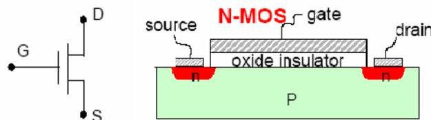
Figure 2. The circuit symbol and structure of NMOS.
