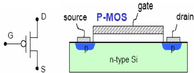
Figure 3. The circuit symbol and structure of PMOS.
