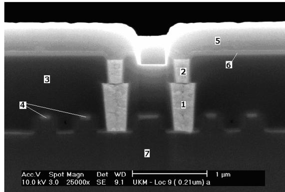
Figure 11. The cross-section of 0.21μm CMOS device. Number 1-7 represent the different locations that have been tested.
