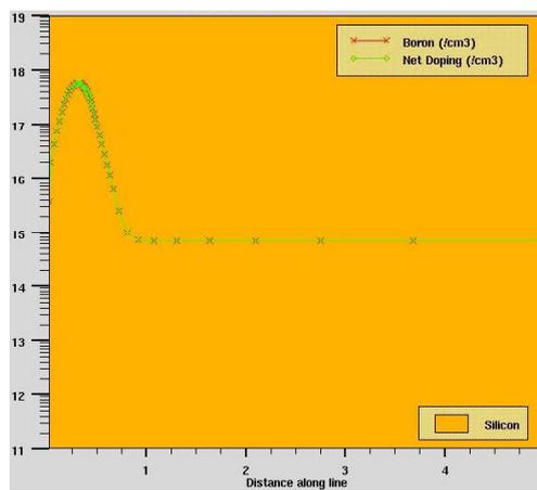
Figure 2. Boron density versus substrate depth of a 0.14  $\mu\text{m}$  NMOS.
