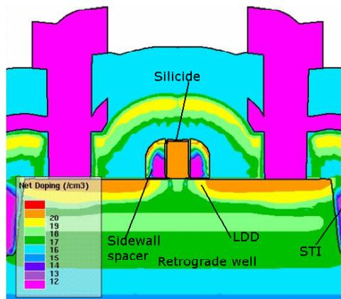
Figure 1. 0.14  $\mu\text{m}$  NMOS.
