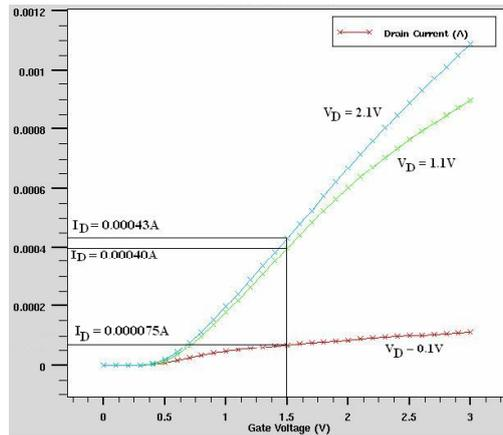
Figure 6. NMOS ID-Vg relationship before metallization 2 is deposited.
