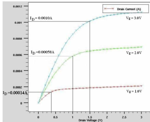
Figure 4. NMOS  $I_D$ - $V_D$  relationship before metallization 2 is deposited.
