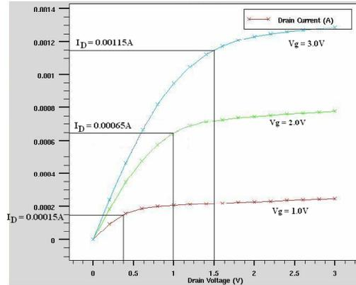
Figure 5. NMOS ID-VD relationship after metallization 2 is deposited.
