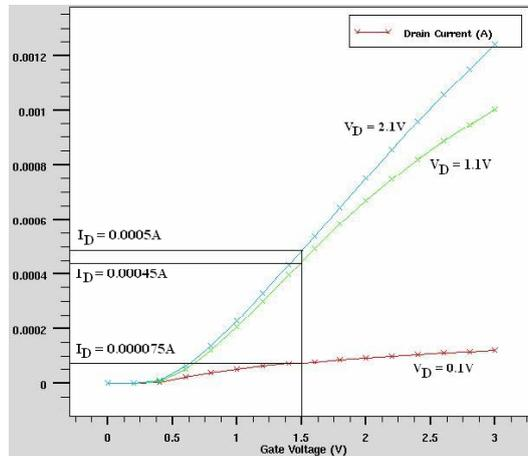
Figure 7. NMOS ID-Vg relationship after metallization 2 is deposited.
