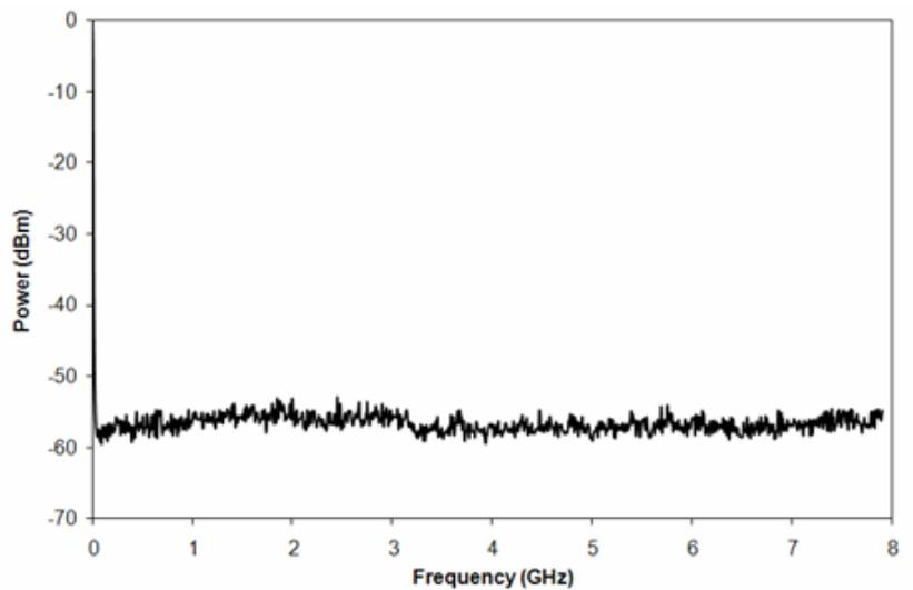
Figure 4 : The frequency spectrum of Brillouin fiber laser from SA of TWF.
