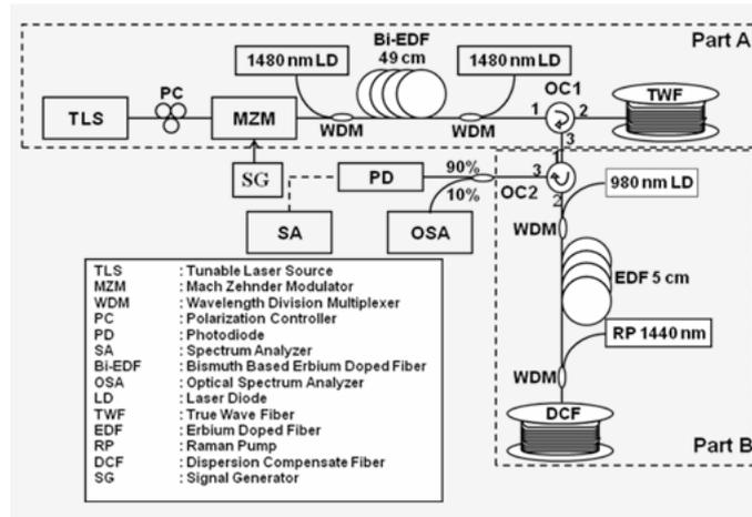
**Figure 1** : Schematic diagram for microwave photonics signals conversion based BSB in optical fiber.
