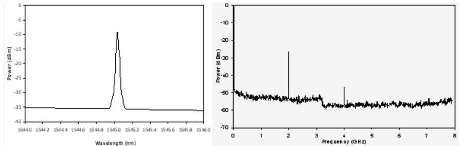
**Figure 2** : The input signal and RF input spectrum for the BP pump.
