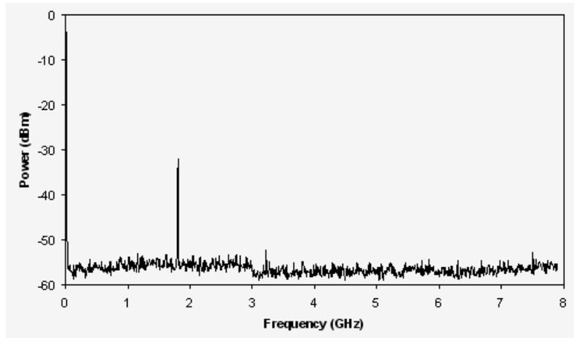
Figure 6 : The frequency conversion of DCF from SA.
