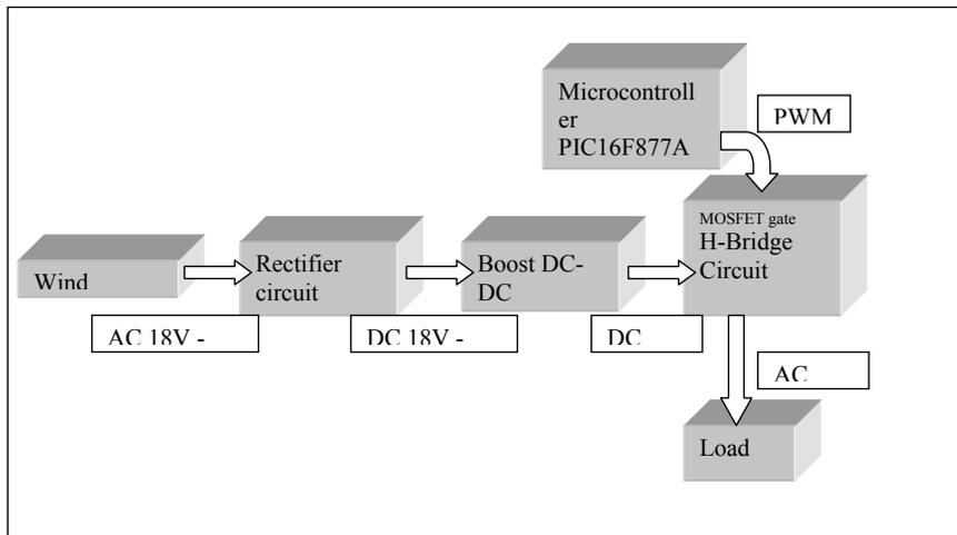
Figure 5: Block diagram of proposed system
