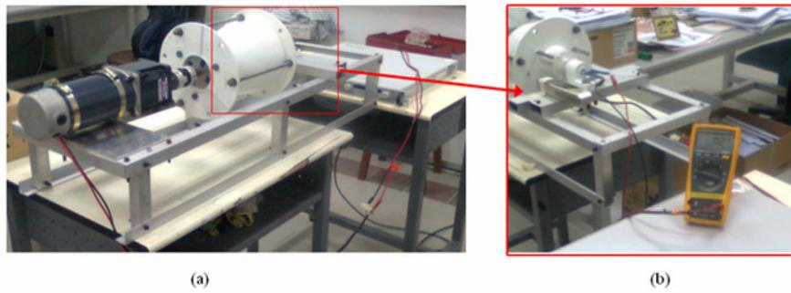
**Figure 10:** (a) Experimental rig for wind generator simulator; (b) Turbine rotational speed and generator terminal output measurement
