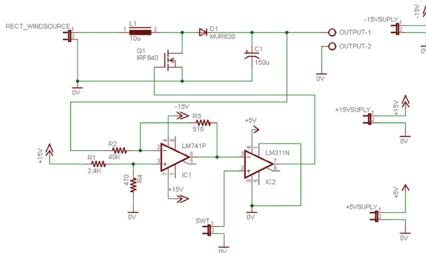
**Figure 7:** Design of Boost DC-DC converter in SIMULINK
