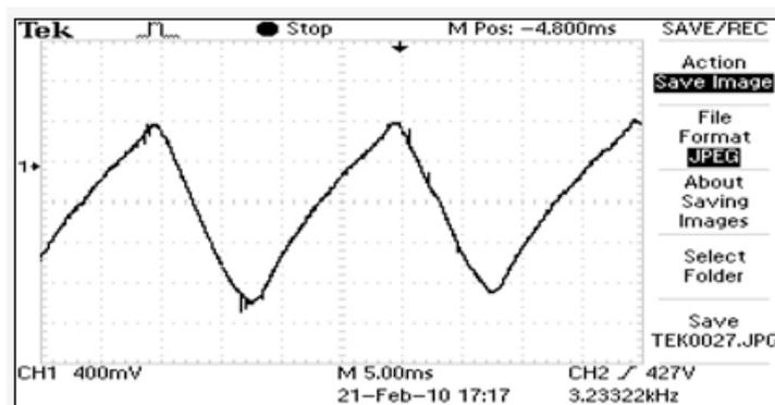
Figure 24: Voltage across resistive load after LC filtering at output of the prototype inverter circuit
