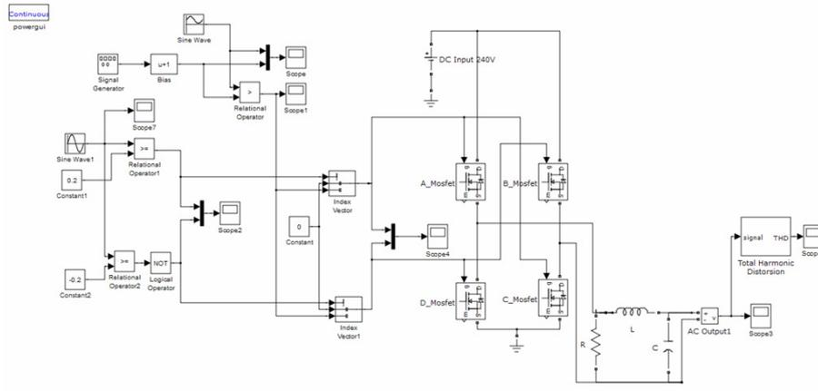
**Figure 15:** Simulation of designed inverter control circuit in SIMULINK
