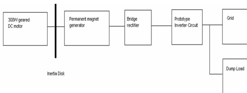
**Figure 9:** Proposed Lab-scale experimental rig
