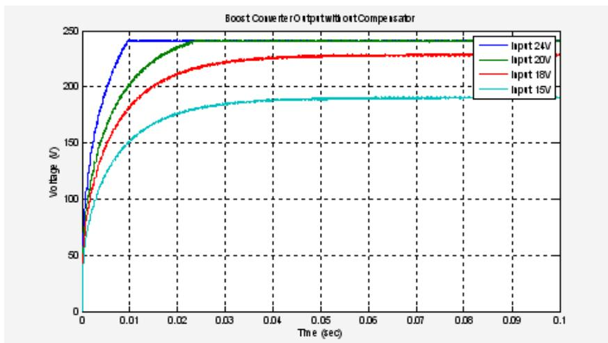
Figure 14: Simulated output of Boost DC-DC Converter
