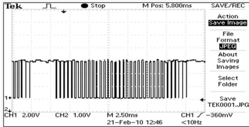
Figure 21: SPWM Trigger signal generated by microcontroller-based prototype board
