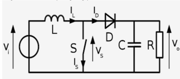
Figure 2: Boost converter schematic
