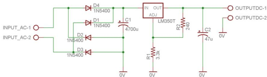
Figure 6: Bridge rectifier circuit
