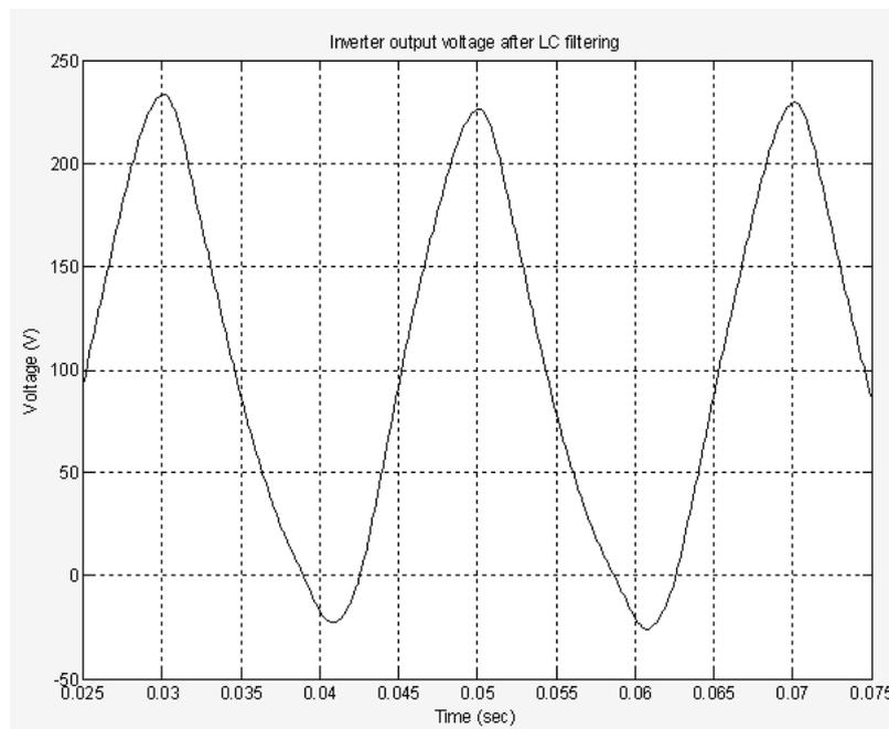
**Figure 20:** Simulated output voltage of inverter circuit after LC filtering
