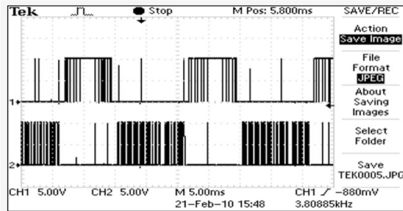
Figure 22: SPWM Trigger signals shown in two channels to the H-bridge gates
