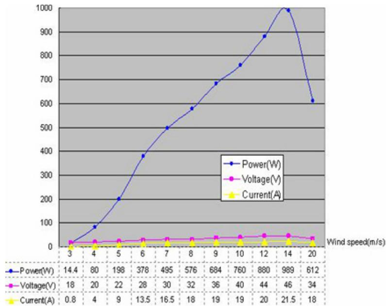
**Figure 11:** 500W Wind Generator Manufacturer Performance Datasheet
