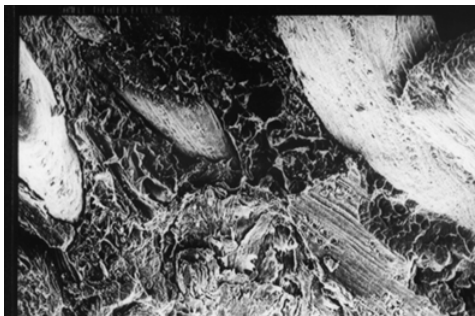
Figure 8 : The SEM Micrograph of Epolene 43 Kenaf Treated Sample
