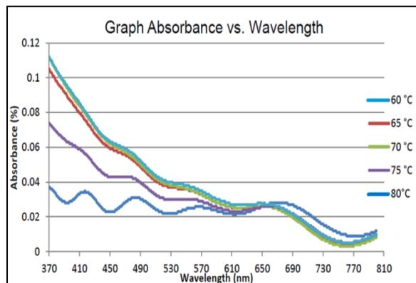
**Fig. 4** UV-Vis absorbance vs wavelength at different water bath temperature
