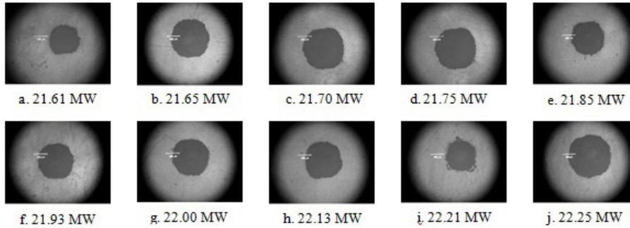
**Figure 3:** Damaged area produced from a combination of long lens system.
