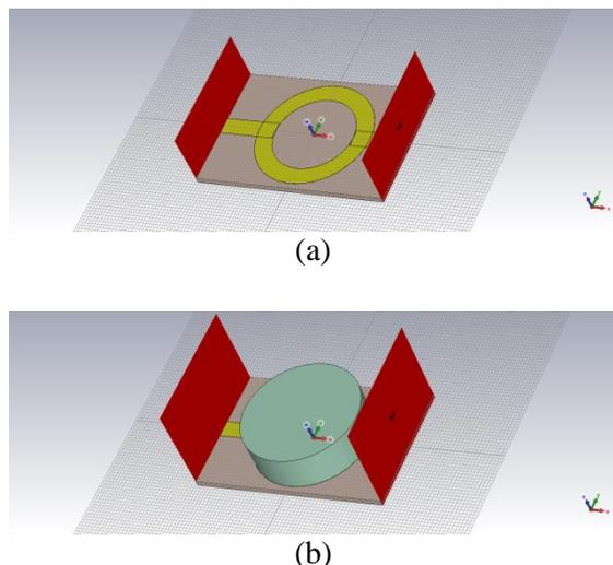
**Fig. 1** The completion model of the (a) unloaded MRR and (b) loaded MRR.
