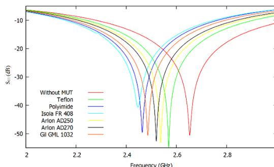
**Fig. 2** Variation of resonant frequency for different dielectric materials and unloaded MRR ( $f_{unloaded} = 2.65340$  GHz).
