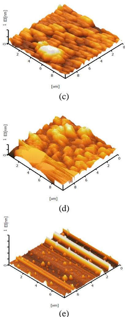
Fig. 1 3-Dimensional AFM images of NiO-YSZ thin film annealing at 600 °C with different layer (a) 1 layer, (b) 2 layer (c) 3layer, (d) 4 layer and (e) 5 layer.
