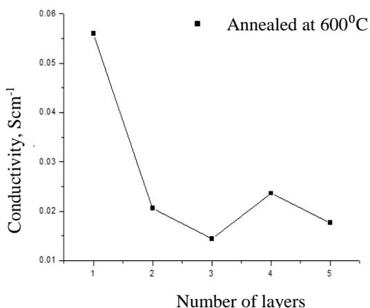
Fig. 2 the graph of conductivity versus number of layers.
