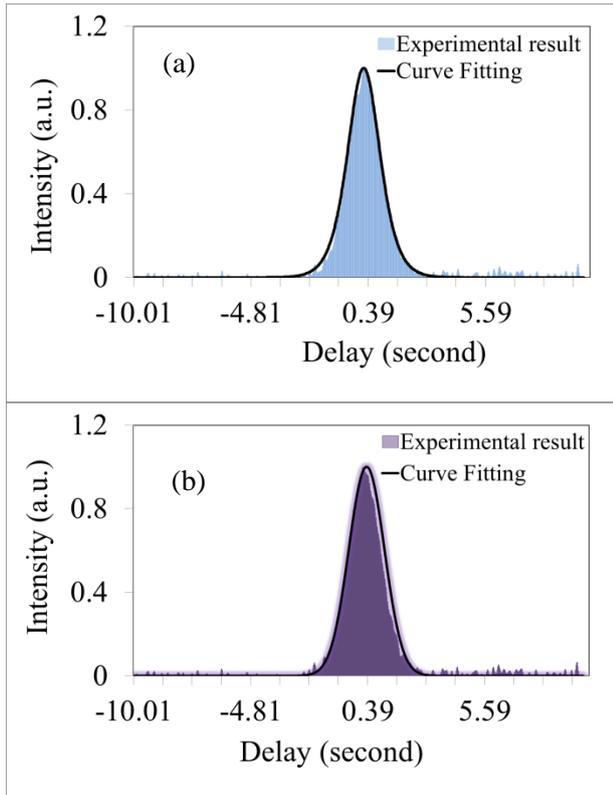
**Fig. 5** The pulsewidth of the mode-locked fiber laser by using (a) M15-EDF and (b) I12-EDF.
