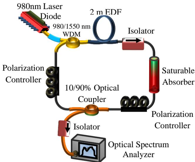
**Fig. 1** Experimental setup of passively mode-locked fiber laser by using D-shaped fiber.
