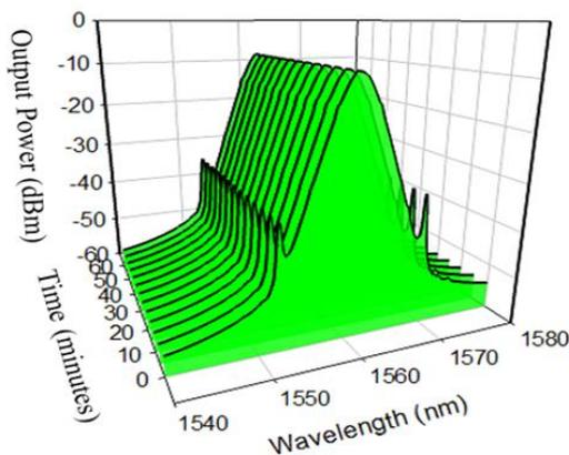
**Fig. 6** Stability performance for the proposed mode-locked fiber laser output.
