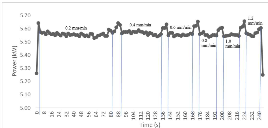
**Fig. 10** Power consumption at multiple feed rate
