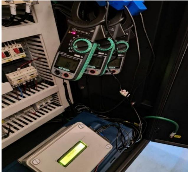
**Fig. 6** Setup for sensor calibration
