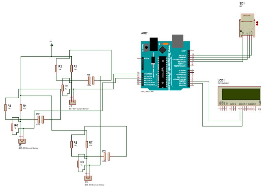
**Fig. 2** Schematic circuit diagram for the proposed energy monitoring system
