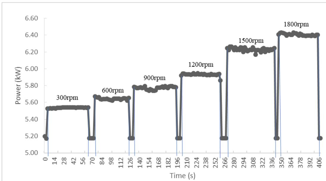
**Fig. 9** Power consumption at multiple spindle rotation speed
