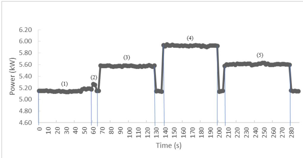
**Fig. 8** Power consumption during machining operation at different experimental stages (in Table 2)
