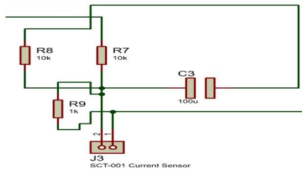
**Fig. 3** Circuit design for current sensor input
