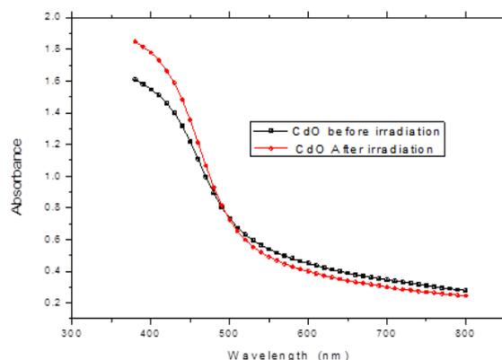
**Fig. 2** Absorbance versus wavelength of CdO thin film before and after irradiated by laser.
