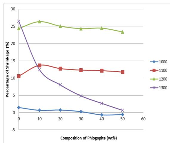
**Figure 1** Graph of the percentage of porcelain shrinkage against composition of phlogopite at different sintering temperatures
