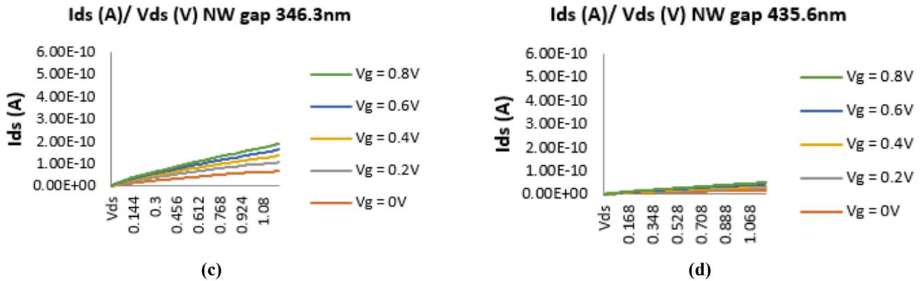
**Fig. 7** Output voltages of the I-V characteristics at low voltages (0-0.8V) for varies nanowire gap (a) Nanowire gap 100.5nm, (b) Nanowire gap 225.8nm, (c) Nanowire gap 346.3nm, (d) Nanowire gap 435.6nm
