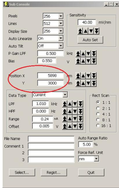
Fig. 2 Auxiliary console window for setting coordinates along the X and Y axes
