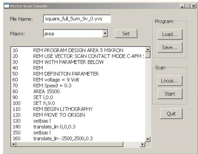
Fig. 3 Loading raster programming in a vector scan console window
