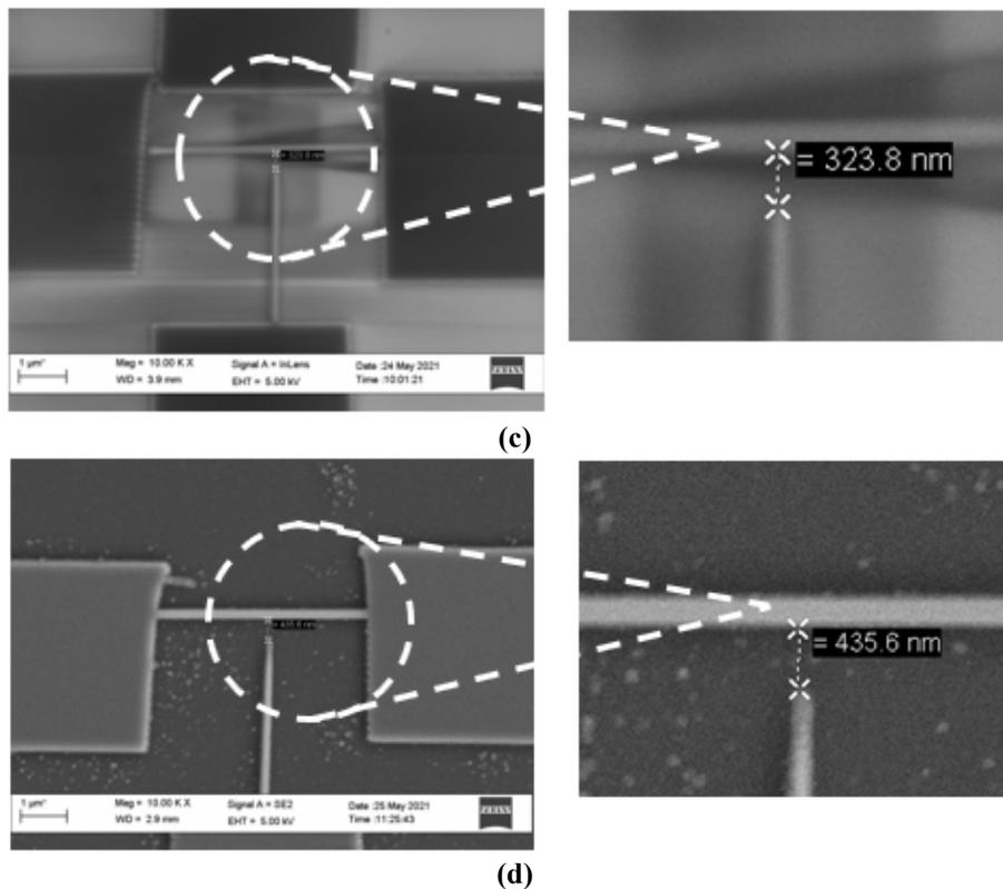
**Fig. 7** SiNWT structure with nanowire gap (c)  $\sim 323.8\text{nm}$ , (b)  $\sim 435.6\text{nm}$
