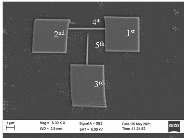
**Fig. 5** Final structure of the SiNWT was fabricated via LAO which developed partial by partial process (partial 1th–5th)
