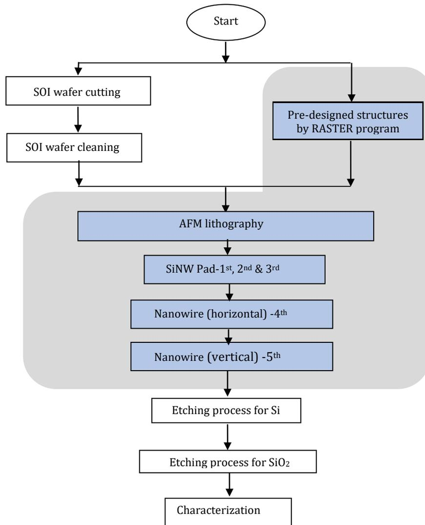
**Fig. 4** The entire process for fabrication of SiNWT
