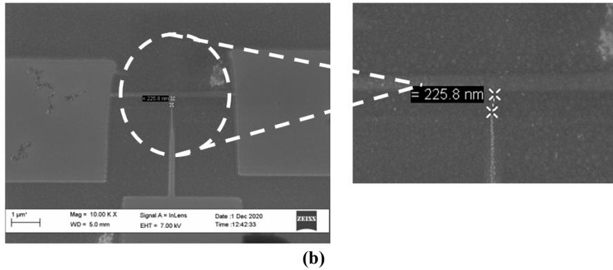
**Fig. 6** SiNWT structure with nanowire gap (a)  $\sim 100.5\text{nm}$ , (b)  $\sim 225.8\text{nm}$
