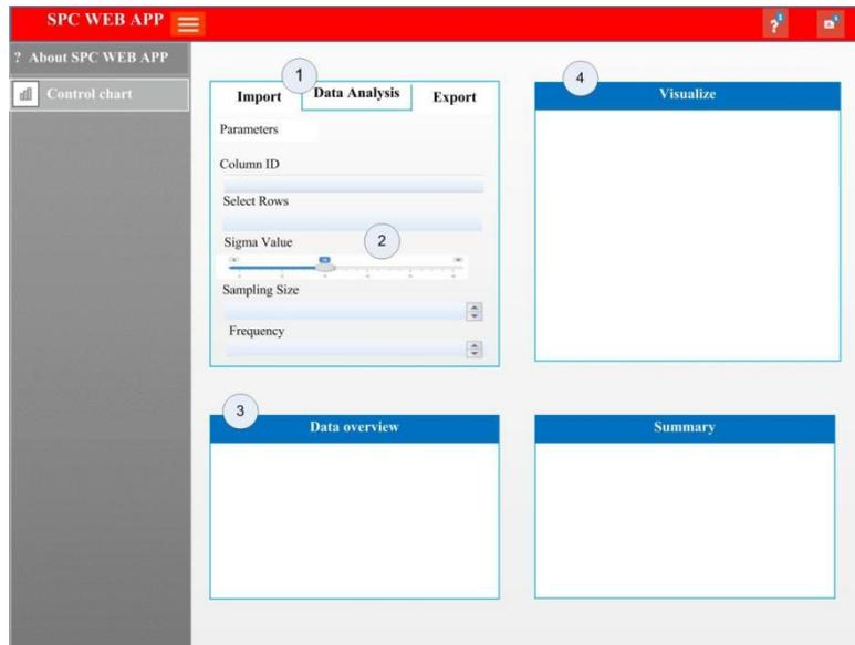
**Fig. 2 - An example of a UI design for an SPC web application: (1) data analysis tab; (2) interactive parameter control; (3) imported raw data overview window; (4) results visualization window**
