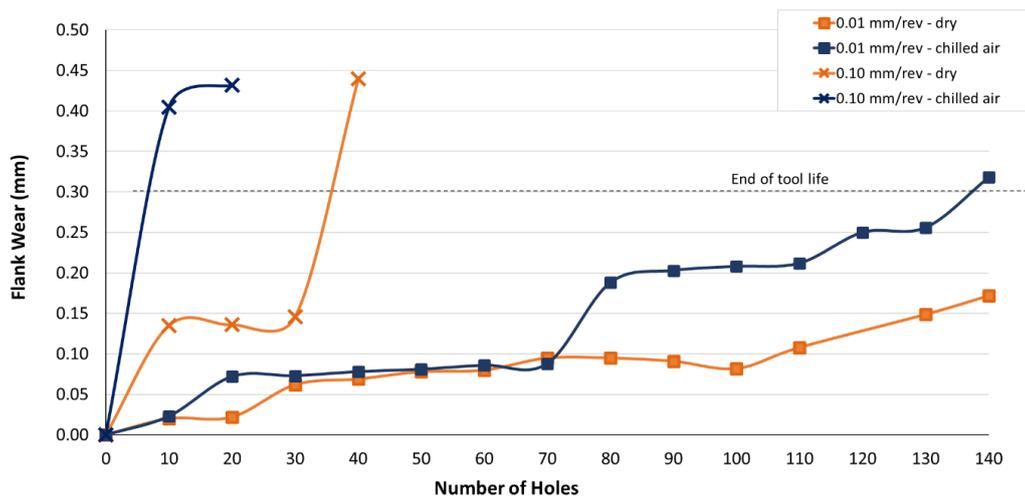
**Fig. 3 - Flank wear when drilling Al 7075 at a constant cutting speed of 123 m/min and feed rates of 0.01 and 0.1 mm/rev in dry and with chilled air**
