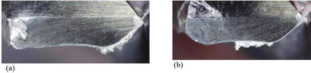
**Fig. 5 - Cutting edge condition after drilling 140 holes at the feed rate of 0.1 mm/rev (a) in dry; and (b) with chilled air**
