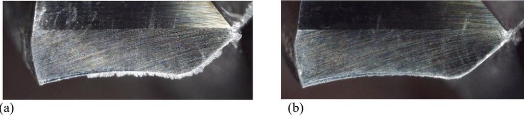
**Fig. 4 - Cutting edge condition after drilling 140 holes at the feed rate of 0.01 mm/rev (a) in dry; and (b) with chilled air**
