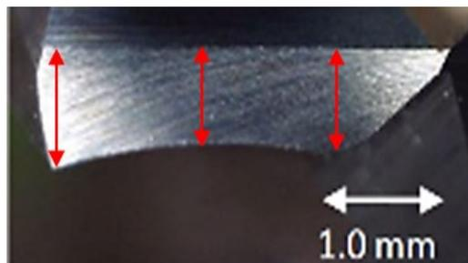
Fig. 2 - Flank face of the drill. The red arrows are the location of wear measurement
