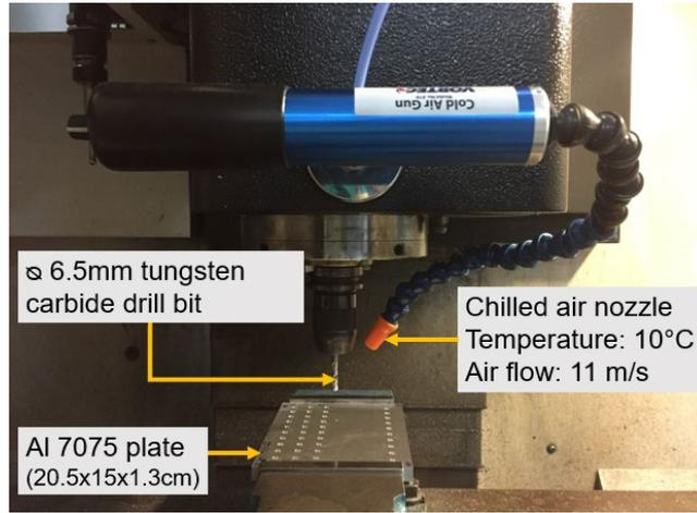
Fig. 1 - Drilling operation setup
