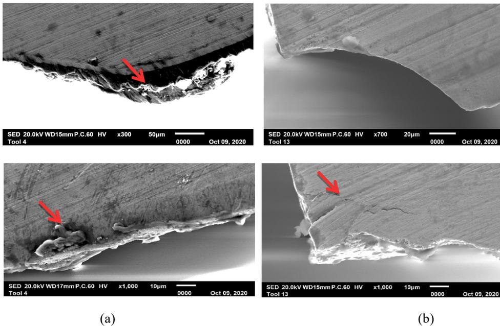
**Fig. 6 - SEM micrographs of cutting tool after drilling 140 holes at the feed rate of 0.01 mm/rev (a) in dry; and (b) with chilled air**
