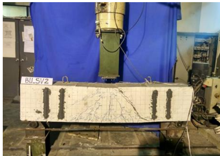
Fig. 6 - BU-SV2 crack pattern
