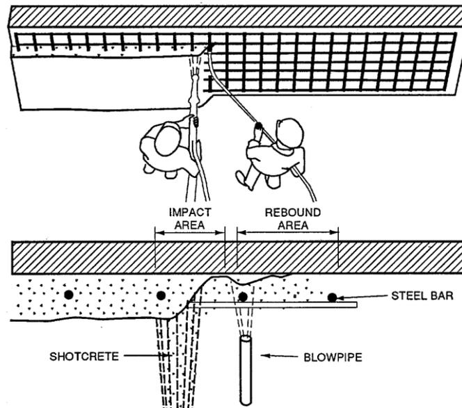
**Fig. 2 - Application of shotcrete to the pre-installed wire mesh (After Gideon, 1993)**
