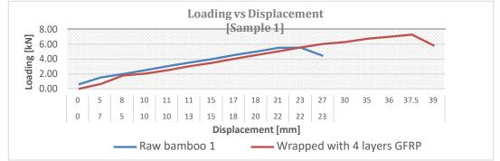
Fig. 6 - Raw bamboo and strengthen bamboo on bending test (Sample 1)
