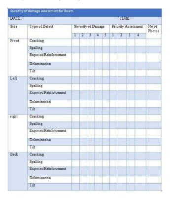
Fig. 4 - Modified assessment form for inspection (PWD, 2002)
