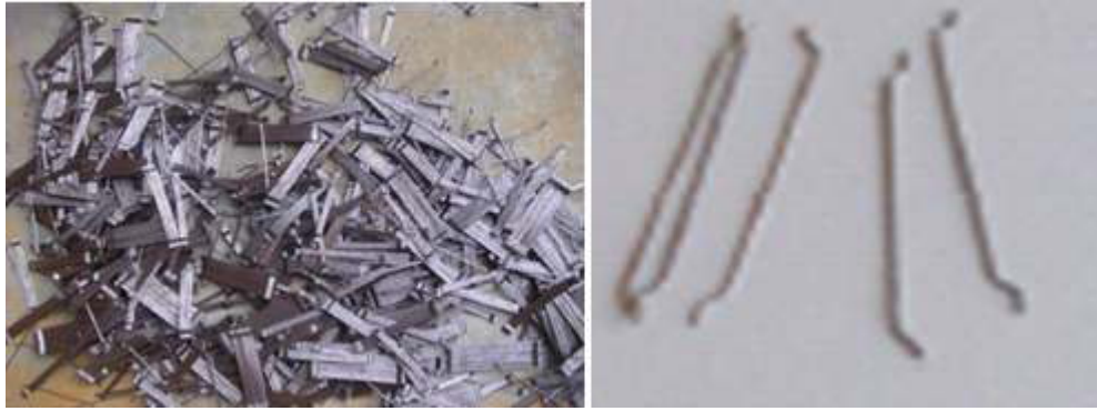
Figure 7: Photos of hooked end steel fibers
