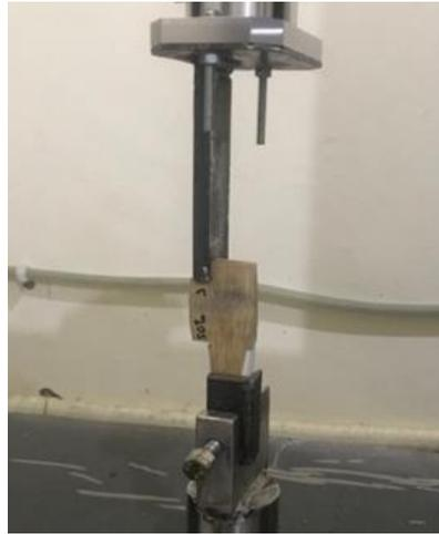
**Fig. 6 - Set up for Shear Test**
