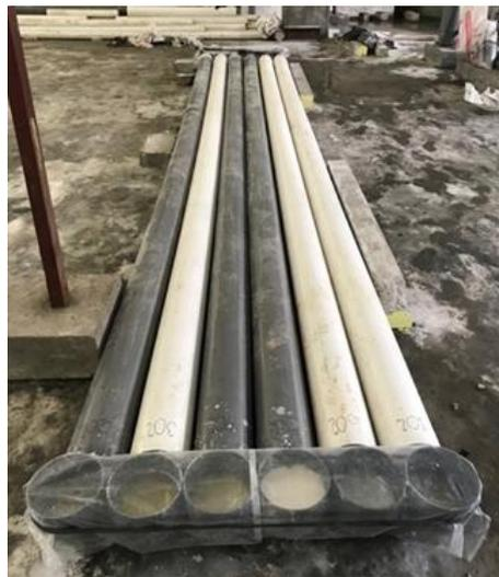
**Fig. 2 - Bamboo soaking process**
