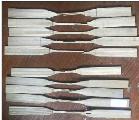
Fig. 13 - Failure pattern of compressive test specimen
