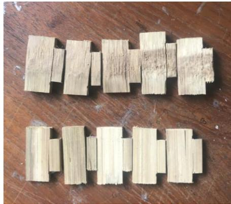
Fig. 15 - Failure pattern of shear test specimen
