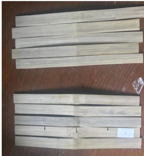
**Fig. 17 - Failure pattern of bending test specimen**
