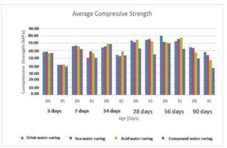
Fig. 4 - Graph of concrete compressive strength test results
