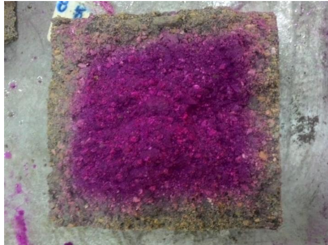
Fig. 5 - The outlook of sliced BSCQD sample after sprayed phenolphthalein indicator solution
