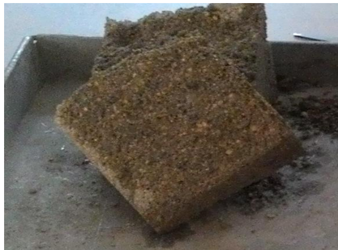
Fig. 4 - The outlook of sliced SCBQD sample before spray phenolphthalein indicator solution
